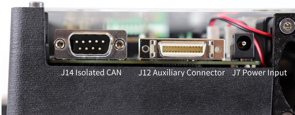
Controller input power supply input utilizes a CUI, PJ-102AH barrel jack connector.
