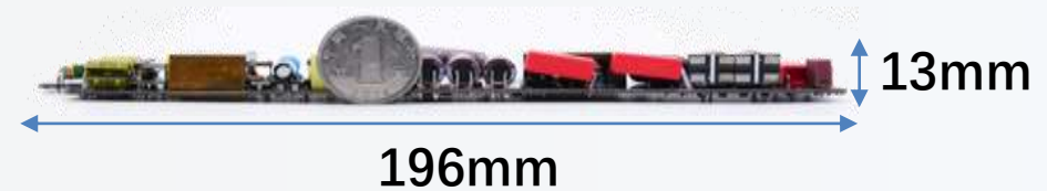
InnoGaN based solution 200W LED driver
