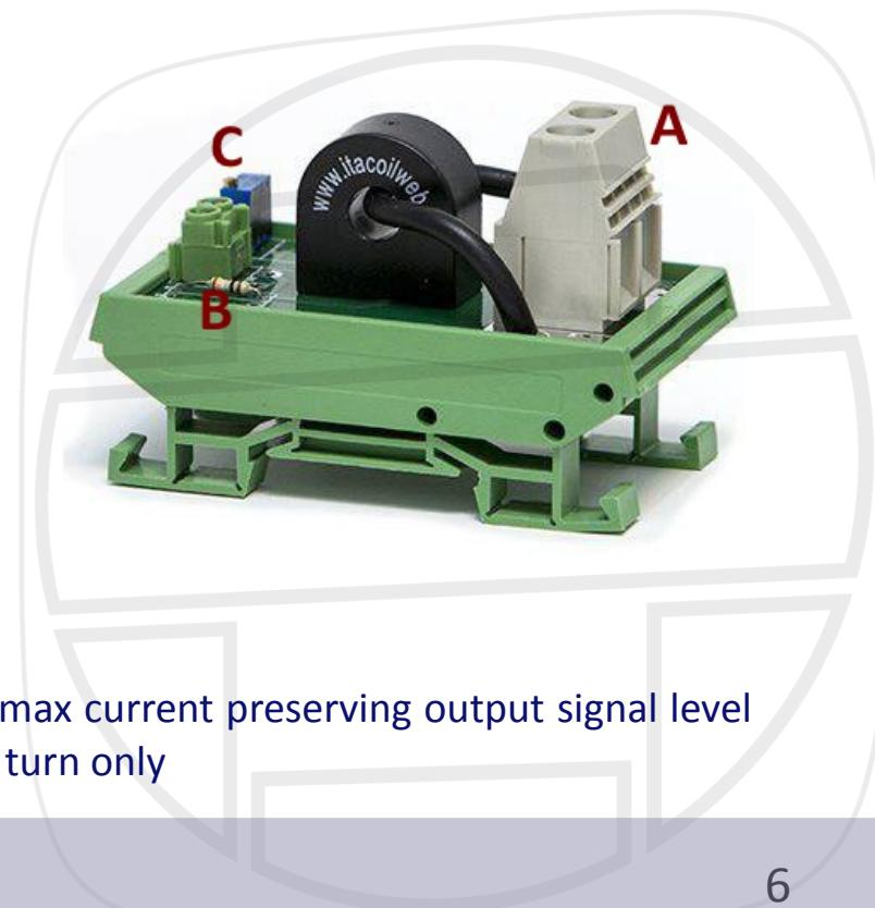
(1) To use a current sensor with currents very lower to its max current preserving output signal level and precision, some primary turns are required instead one turn only
