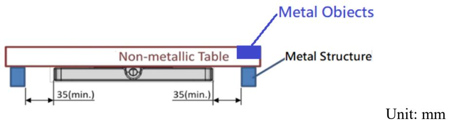
If there are unmovable metal objects inserted on the non-metallic table, there shall be at least above 35mm safety distance between the wireless charger and the metal objects.
