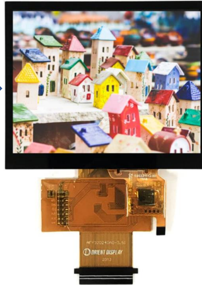
AFY320240A0-3.5IN TH-C 3.5" LCD with Touch
