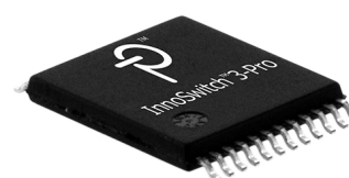
Figure 2. High Creepage, Safety-Compliant InSOP-24D Package.
