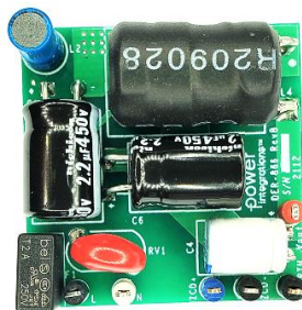
RDK-866 5V/500mA output Non-isolated ZCD LNK3307
