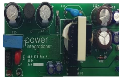
DER-879 12V/0.75A & 5V/0.2A ZCD + Xcap discharge LNK3317
