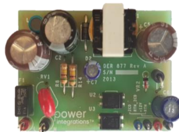
RDK-877 12V/0.5A output Isolated ZCD signal LNK3306
