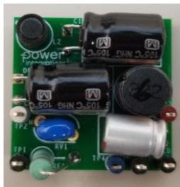
DER-874 6V/80mA output <150uA input current LNK3302
