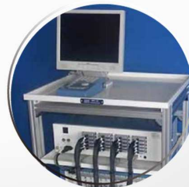
OLED Lifetime Tester
