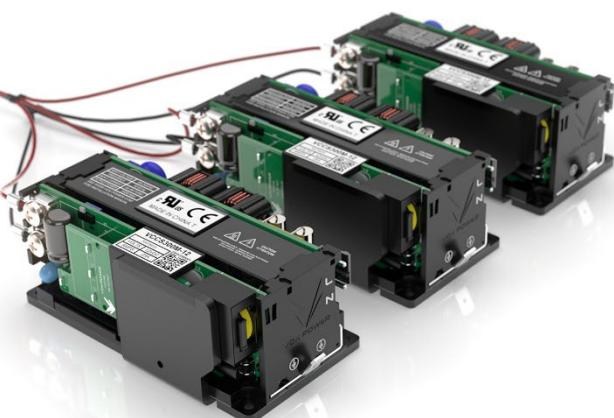
This product series offers power densities exceeding 23W/in<sup>3</sup> with efficiencies up to 95% in a scalable power architecture. Power solutions of 300 Watts, 600 Watts, 900 Watts and beyond can be achieved by using the onboard droop current share function, which allows end users to scale up or down depending on their power requirements.
